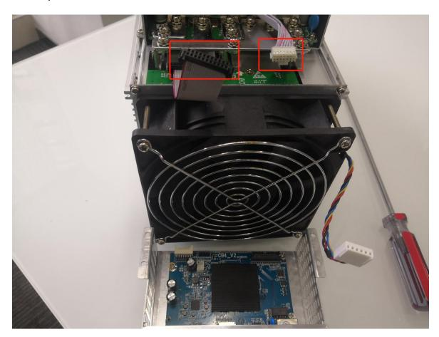
3) Remove the four screws fixed on the bracket and take out the control panel from the bracket as shown:
