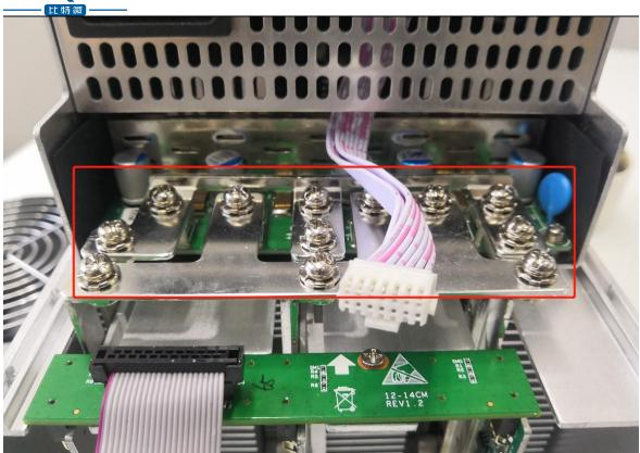
4) After the copper row is installed, the control board and the fan are installed, and the hash board is installed, as shown:
