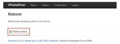
After restarting for about 30s, the machine system will automatically jump to the login interface.
