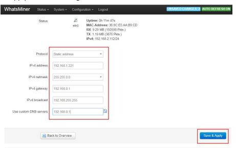
After saving the application, you need to re-use the newly set static IP address to log in to the mining machine (otherwise the page will display loading until the loading fails).
