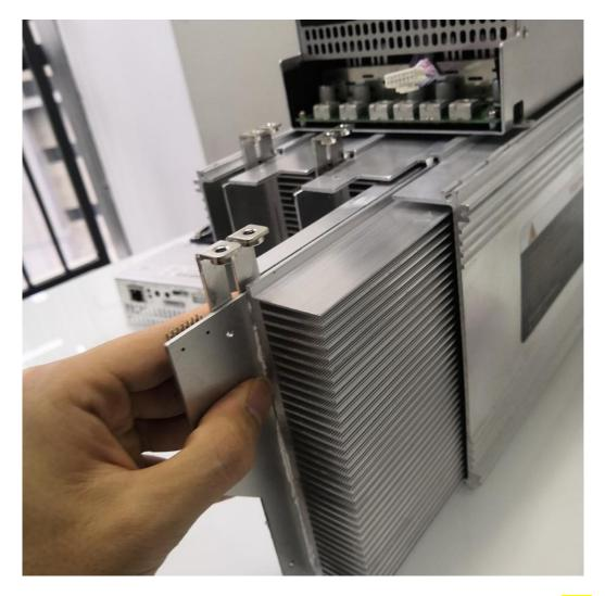
2) After installing the hash board into the chassis, first install the adapter board. The socket of the adapter board and the pin of the hash board must be installed in place to avoid other problems caused by contact problems, as shown:
