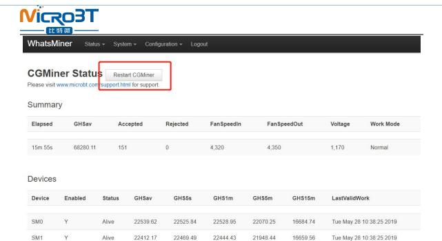
(4) Restart the control board and check whether the configuration modification takes effect. (If you do not choose to restart cgminer, after the configuration is modified and saved, you can also restart the control board to make the configuration take effect.)
