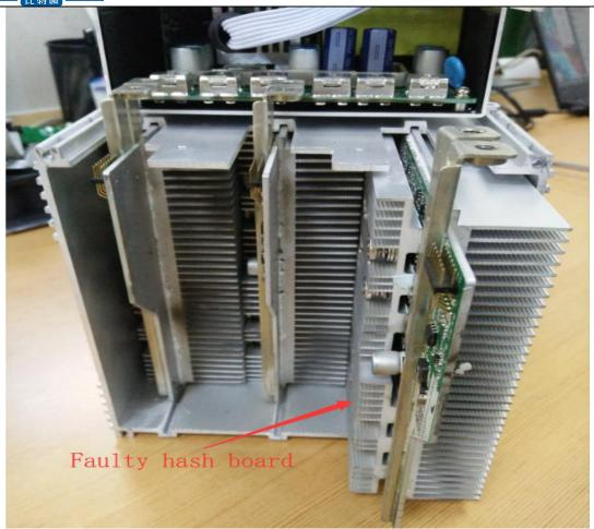
4) After taking out the hash board, record the serial number above or use WeChat "sweep" to scan the power board serial number and provide it to the relevant aftersales technician, as shown:
