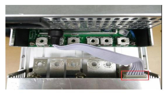
2) Then connect the 6 positive and negative terminals on the power supply to the copper row one by one, and then install 6 screws in turn. The screws should be tightened and the gasket should be aligned parallel to the edge of the copper bar to avoid short circuit burning the power supply or the power board, as shown below:
