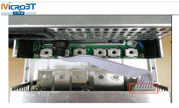
2) Then connect the 6 positive and negative terminals on the power supply to the copper row one by one, and then install 6 screws in turn. The screws should be tightened and the gasket should be aligned parallel to the edge of the copper bar to avoid short circuit burning the power supply or the power board, as shown below:
