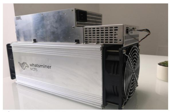
Whats Miner M21S Blockchain Server Artifact Product ParameterIntroduction as below: HashRate: 56TH/s ±5% Power: 3260W±10% Power Rate: 60W/T Power Supply: WhatsMiner Power Supply P21 (220,3500W±10%) Environment Temperature: -5℃~40℃ Product Size: 390mm\*155mm\*240mm
