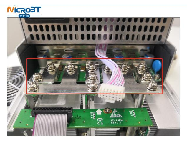
4) After the copper row is installed, the control board and the fan are installed, and the hash board is installed, as shown:
