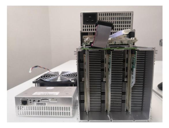
2) Remove the adapter plate and the copper bar fixed to the control panel as shown:
