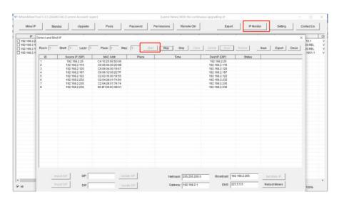
After IP detection is completed, you can click on the [Save] button to save the current data, close the window and do not disappear, or the [Export] button to export the current mine IP list to the file.
