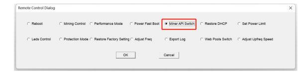
After opening the API switch, you can use the API interface to obtain various states of the miner and modify the parameters of the miner.
