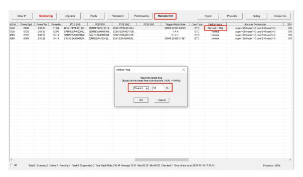
After the operation is completed, the selected machine displays the percentage of up / down actions corresponding to [performance Mode].
