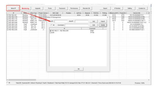
Enter the corresponding IP segment in the Start IP and End IP input fields, and then click Add.
