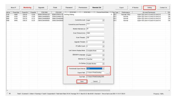
After the operation is completed, the tool data file is saved to the corresponding export path according to the selected export interval.
