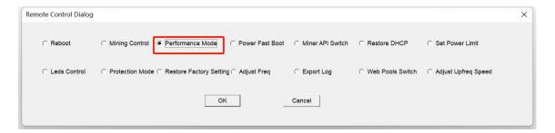
After selection, a pop-up window will pop up. Select one and press Select to switch the force calculation mode. Note: at present, the high-performance mode only supports m30s series and the voltage requirement is more than 230V, as shown below:
