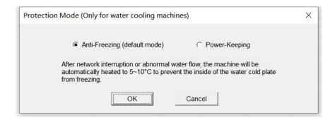
Switch the power-Keeping mode, and the machine will continue to work to maintain the power after the disconnection; if the water flow is abnormal, it will automatically switch to the anti-icing mode, as shown below:
