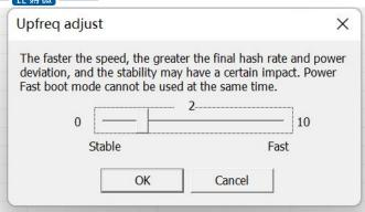
Frequency adjustment range:  $[0^{\sim}10]$ ; function: 0 indicates normal frequency search speed. The larger the number is, the faster the frequency search speed is. Stability may have an impact.
